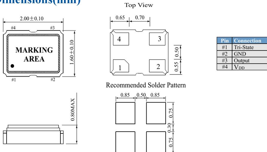
\*\*Note: 0.01uF bypass capacitor should be placed between V<sub>DD</sub>(Pin4) and GND(Pin2) to Minimize power supply line noise
